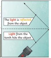
Surfaces that best reflect are smooth and shiny. Mirrors reflect light very well, so they create a clear image. An image in a mirror appears to be reversed. For example, if you looked in the mirror and raised your left hand the mirror image appears to raise your right hand.
